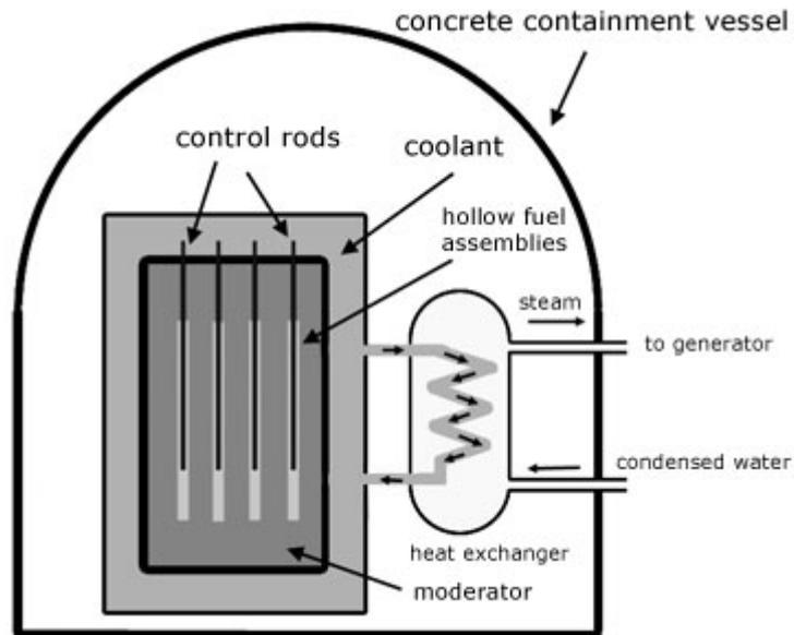
Ideally fission should proceed at the rate of one fission for one neutron produced. The trouble is that in the process two and sometimes three neutrons are produced. To limit the numbers of neutrons in the reactor **control rods** are used. These are rods of boron-coated steel which absorb neutrons. When the rods are raised from the reactor, neutron numbers increase. When they are lowered, neutron numbers decrease. In this way the rate of fission is controlled.
